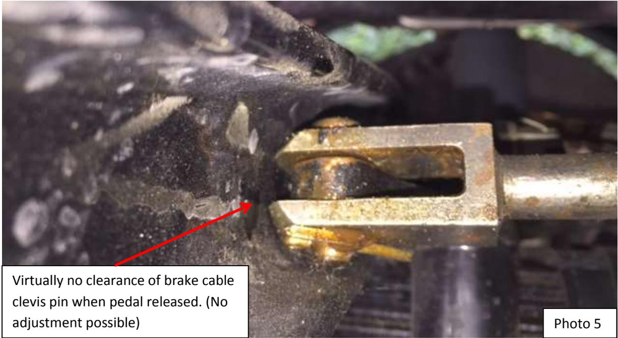
Virtually no clearance of brake cable clevis pin when pedal released. (No adjustment possible)
