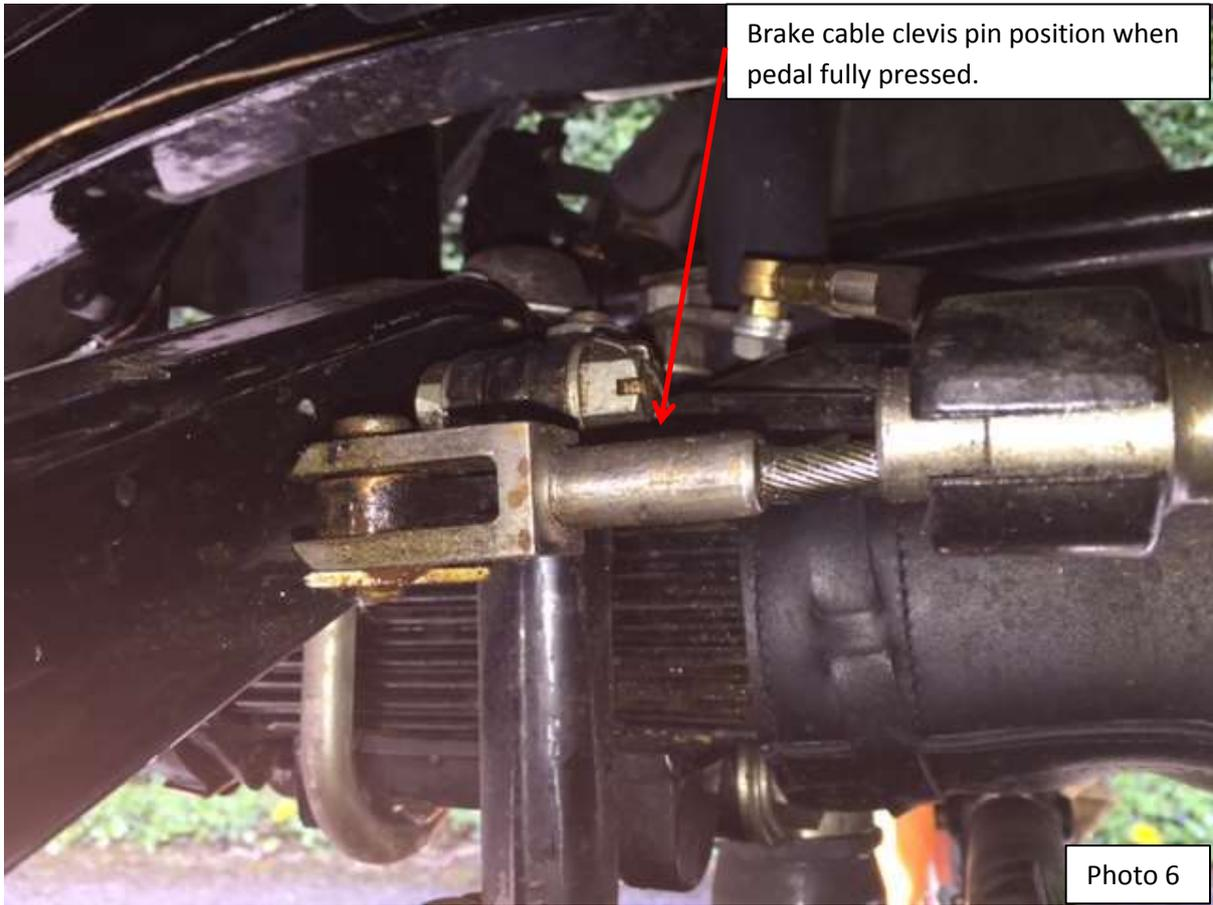
Brake cable clevis pin position when pedal fully pressed.
