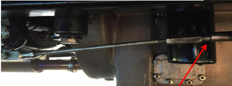
Clearance of brake rod when pedal released approx. 10mm
